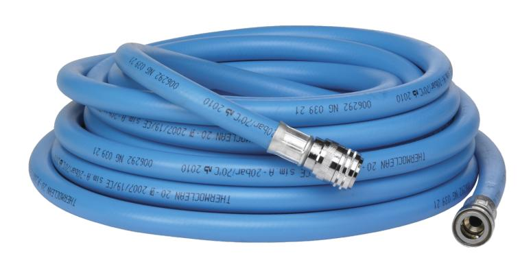
This Hot Water Hose is ideal for cleaning with water up to 70° C. It is equipped with a 1/2" Q-coupling in both hose ends. Water tap nipple, 0700 provided for 1/2", 3/4" and M22x1 screw thread types. Can be used with the following Vikan Q-couplings 0700, 0705 and 0712 as well as other Vikan products equipped with a 1/2" Q-nipple.
