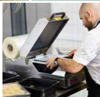
2. Pull the film with two hands over the tray.
