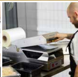
4. The machine opens automatically once the tray is sealed (except manual machines DF10/15).
