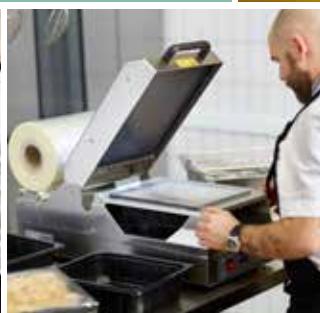
3. Push the lid of the machine down until it starts to seal.
